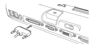
Figure 4-17. Connecting a Parallel Device to Port Replicator
